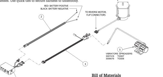
**CONTROLLER WIRES** INPUT WIRES: RED (10AWG) - BATTERY "+" BLACK (10AWG) - BATTERY "-" BLACK - SPINNER NEGATIVE RED (16AWG) - IGNITION "+"
